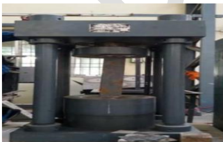
Figure-1. Specimen in compression testing machine for testing.
