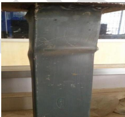
Figure-4. Buckling of 28 day specimen.
