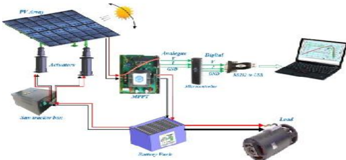
Figure 5: Solar Panel Interfacing With Micro Controller
