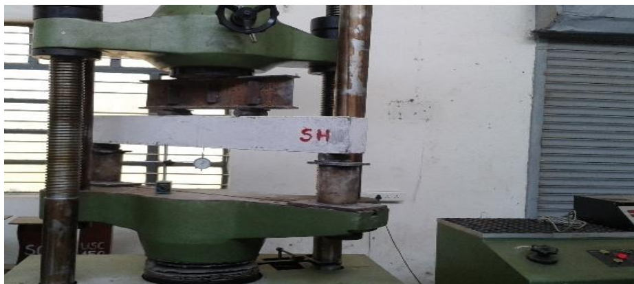
Figure 5.4 Testing of beams
