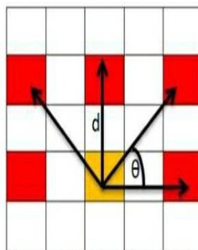
Fig.4.1 The Co-occurrence for one pixel (yellow pixel) with  $d=3$  and  $\theta \{0, \pi/4, 2\pi/4, 3\pi/4\}$ .
