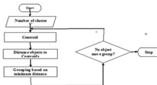
Figure 5.1: Flowchart of K-means clustering
